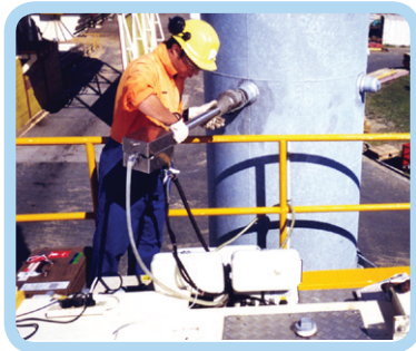
A technician secures a sampling assembly into a stack
